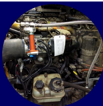
H2 injection manifold in-line with air intake blends H2 and air before entering engine block, NO engine modification.
