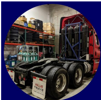
H2 gas handling components behind or under cab.
